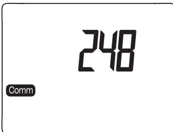
The meter address contains 3 digits, and can be any one from 001 to 255.
